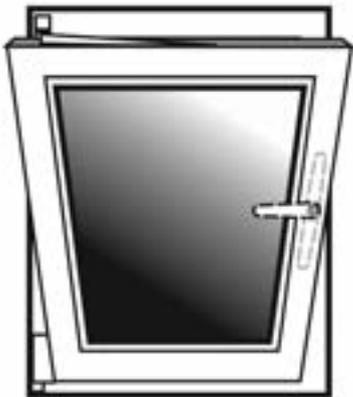
The term 'Tilt-Turn' refers to the sequence of operation of the window which is designed for safety, to initially select the 'Tilt' mode, followed by the 'Turn' mode.
